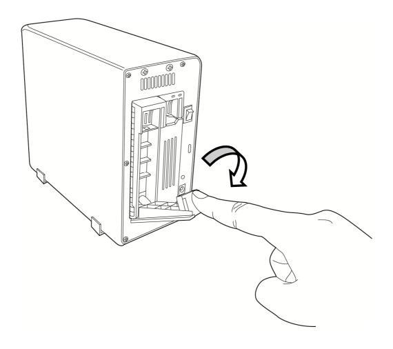
3. Hold the HDD enclosure and pull it out.
