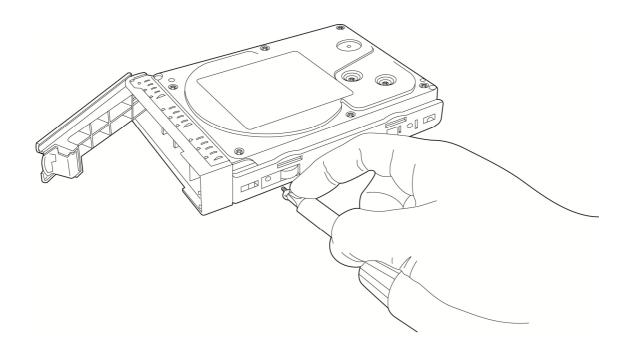
7. Press the top of HDD enclosure and fully push it back into NVR, as instructed (do not press white lever back now, and it should remain in open position in this step).
